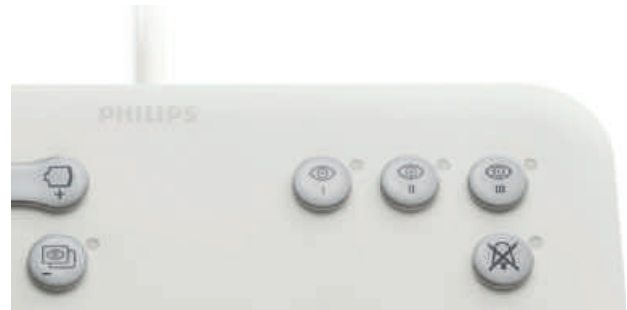
Figure 13: Position and labeling of the three fluoroscopy flavors on the user interface of the AlluraClarity and Allura Xper systems
