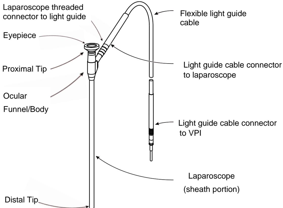
**⚠ WARNING:** Both ends of light guide cable and distal end of laparoscope can become hot and may cause patient/operator burns or thermal damage to surgical equipment (e.g. surgical drapes, plastic material, etc). Do not touch the glass tip of light guide cable or distal end of laparoscope. Do not allow the glass tip of light guide cable or distal end of laparoscope to contact the patient, surgical drape, or any other flammable material.
